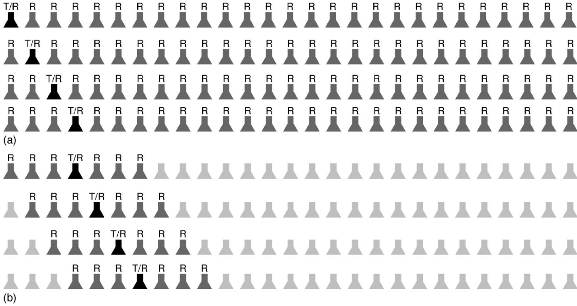
FIG. 5. Full aperture and subaperture processing. (a) In full aperture processing, the time series measured at all receivers are processed together. (b) In subaperture processing, the data from a shifting subarray consisting of a transmitter/receiver surrounded by an equal number of receivers are processed together.
